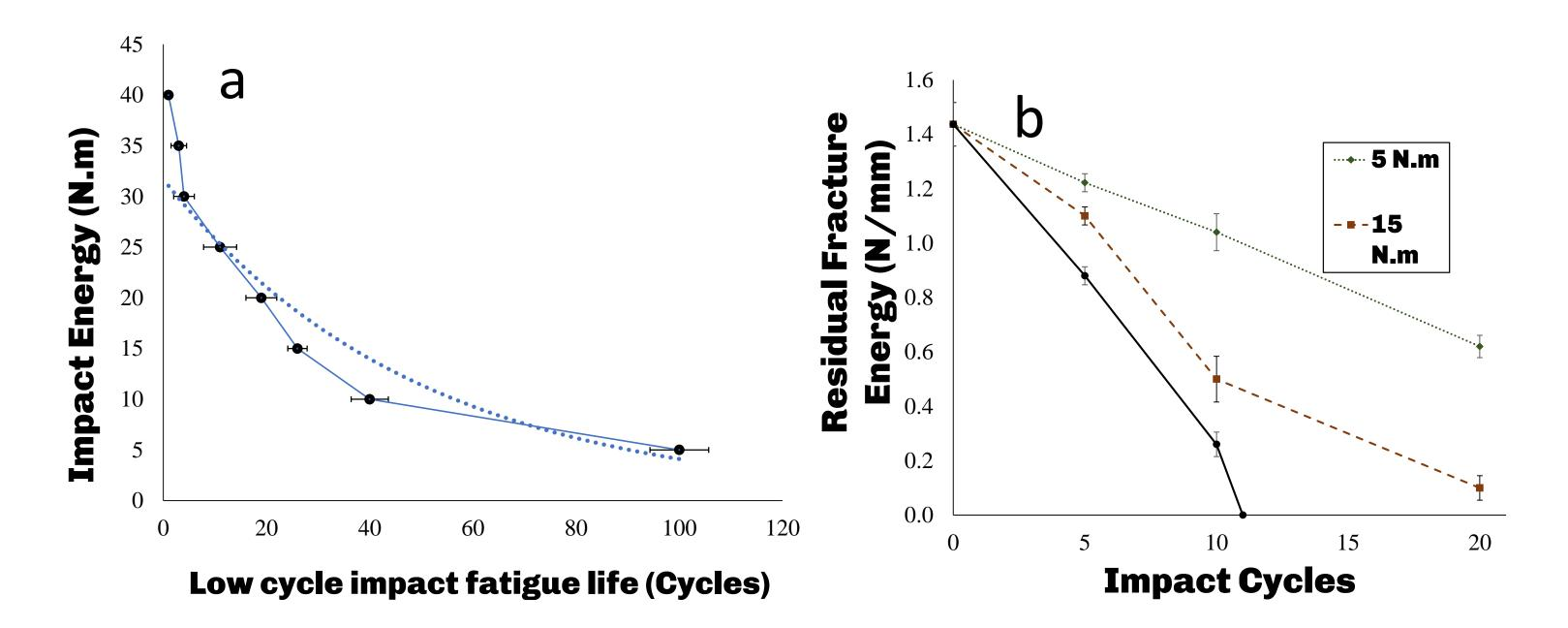
Figure 3 – (a) Impact fatigue life of the ENF joints; (b) Residual fracture energy as a function of the number of impact cycles
