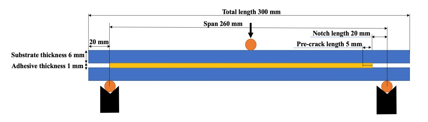
Figure 1 - ENF specimen geometry
