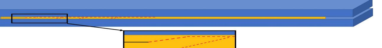
Figure 4 – Crack propagation path along the bond line
